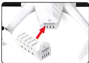
2.1.1 Install the fully charged battery DO NOT turn on the battery until later. *Please check the charger manual for charging instructions
