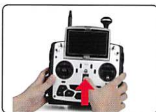
2.1.3 Put all function switches to 0 position, put all trims/knobs on Mid position, move the throttle to the lowest position, then turn on the radio power.
