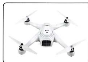
1.4 Propellers assembled (unassemble skid landing)
