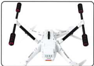
2.1.5 Turn the aircraft to its UP-right position.The Red LED flashing will stop shortly.When it stops, the DEVO F12E and the X4 have successfully connected to each other. * This process is called "ID binding"
