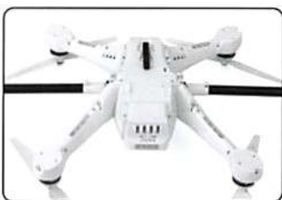
2.1.2 Turn X4 on its back. The belly and the retractable legs should now be facing up. MAKE SURE nothing is blocking the legs.
