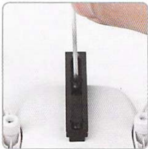
3.1 Use 2 M3X8 screws to install the Gimbal fixing block into the bottom of the fuselage.
