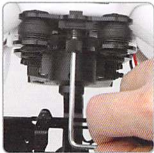
3.3 Fix the spring into M3x12 screw, then align the screw with the threaded hole and tighten to fix the Gimbal.
