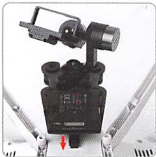
3.2 Align the Gimbal chute with the fixed block, then install it into the bottom of fixing block in the direction of the arrow.
